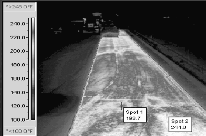
TEMPERATURE DIFFERENTIAL - MAT w/PAVER
